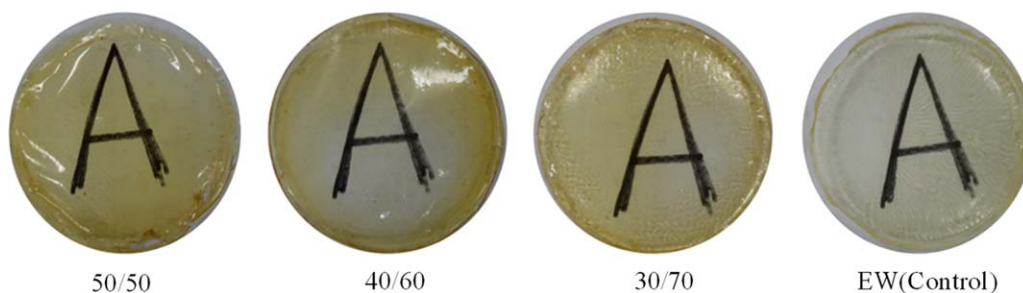
Figure 4. Images of AG/EW films obtained by casting method. [Color figure can be viewed in the online issue, which is available at wileyonlinelibrary.com.]
